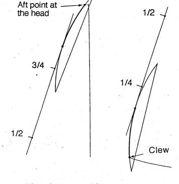
When the pattern is positioned according to the instruction above, the leech shall not project outside the pattern between the points of positioning.
