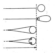
If the luff is set in a luff groove, the width at the head, the 'B' measurement and the cross widths shall be taken to the aft edge of the mast.
